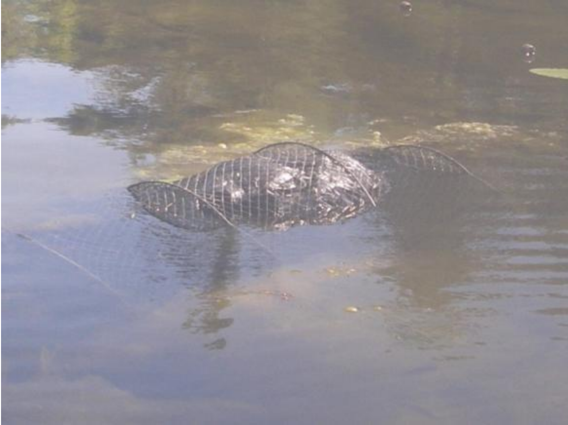
Figure 5-2. A hoop net breaches the surface through the use of floats (i.e., water jugs and Styrofoam in a black garbage bag).
