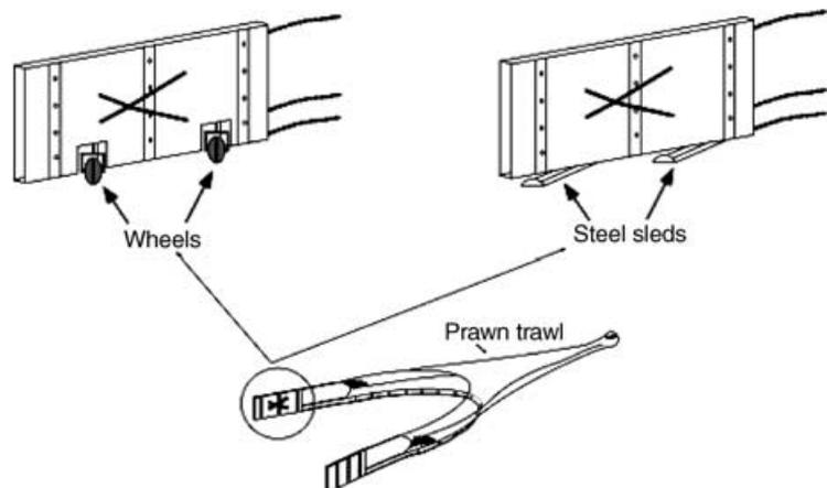
**Figure 9** Two options that may reduce the ecological impacts of otter boards – using wheels and angled sleds on the base of boards.
