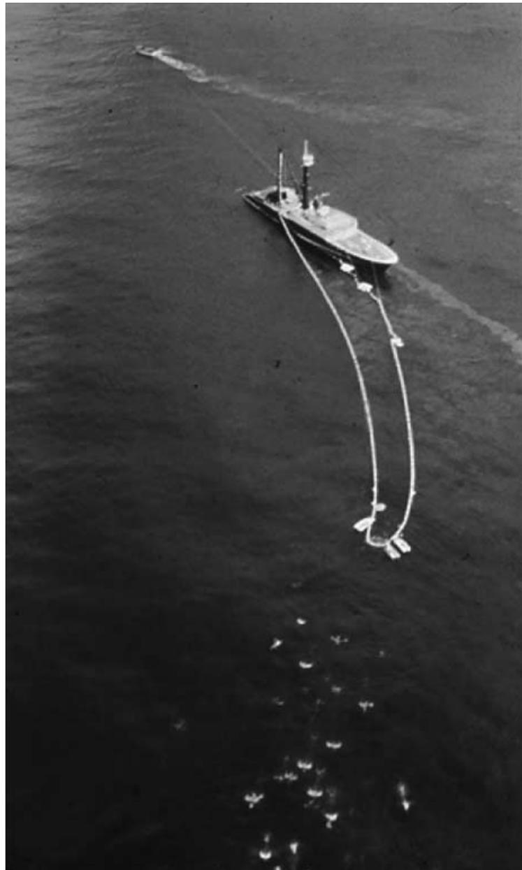
**Figure 4** The 'backdown' manoeuvre used in tuna purse-seining.
